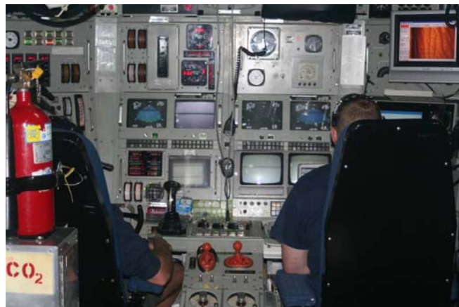
Figure 10. The controls and sonar equipment. (George Schwarz)
