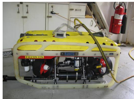
Figure 7. The SeaEye Falcon, a remotely operated vehicle used in 2007. (M. Ryan)
