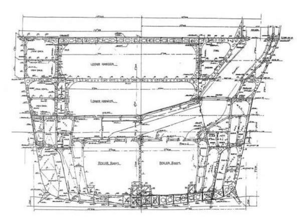
Because this image includes numerous dimensions, it is fairly simple to measure and compare lines that are supposed to be of identical or similar lengths. The hull outline below the waterline should be symmetrical about the centerline but actual measurements show otherwise.
