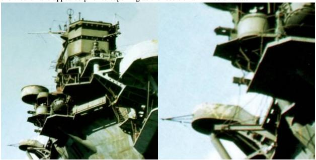
As expected, details of the rotated image are easier to recognize. It is particularly interesting to notice the gun tub in the lower left of the picture. There appears to be a metal beam tied in place with rope and helping to support the platform. This is possibly an interim repair following an earlier air attack.
